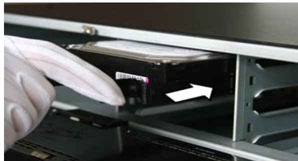
Figure 2-14 Insert HDD to the Slot
