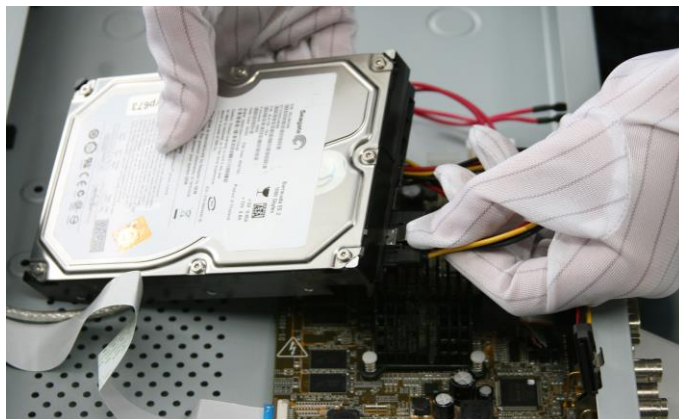
Figure 2-10 Connect Power Cable
