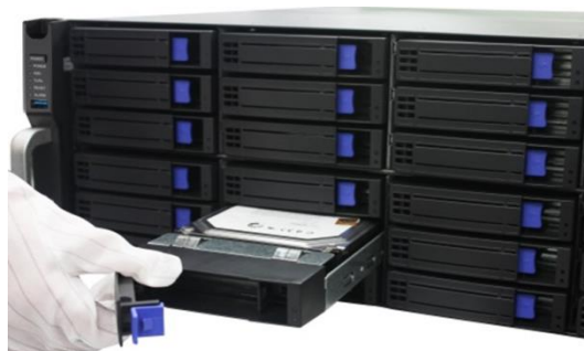
Figure 2-5 Push the Dummy HDD into the Slot
