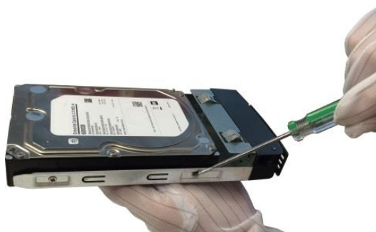
Figure 2-4 Fix the Hard Disk
