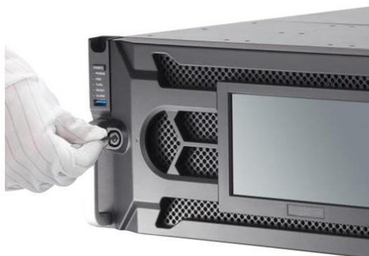
Figure 2-1 Unlock the Panel
